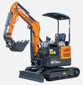
1.7-ton electronic excavator (DX20ZE)
